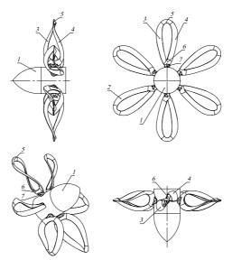
Fig. 1. Tandem propeller with jointed blades by tip vortex generator
