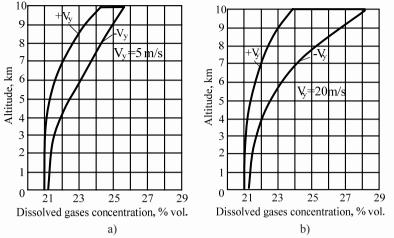
Fig. 5. Change of oxygen concentration in the space above fuel as the aircraft tank is risen to the altitude and at 70 % fuel tank filling
