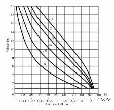
Fig. 2. Theoretical dependence of oxygen concentration in the space above fuel from the volume of the tank filled with fuel and altitude of an aircraft:  $I - O_2 - 33$  %;  $2 - O_2 - 29$  %;  $3 - O_2 - 27$  %;  $4 - O_2 - 25$  %;  $5 - O_2 - 23$ %;  $6 - O_2 - 22$  %
