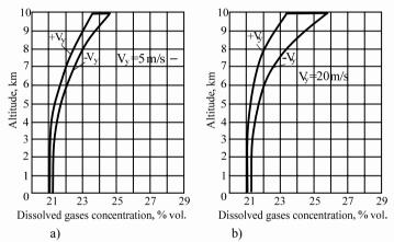
Fig. 4. Change of oxygen concentration in the space above fuel as the tank is risen to the altitude and at 40% fuel tank filling
