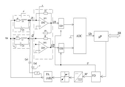
Fig.1 Functional scheme of the measuring channel.
