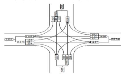
**Fig. 1.** Scheme of the traffic direction of the traffic intersection.
