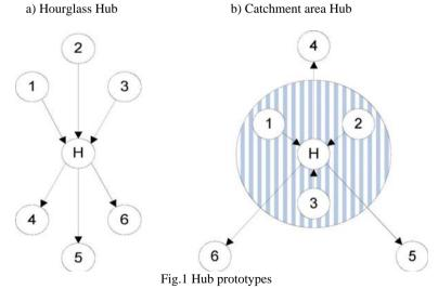
The hourglass hub depicts a typical north-south (could also be West-East) passenger stream which is bundled in the hub for distribution to southern
