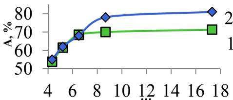
Figure 1 – Dependence of the removal efficiency of sulfate ions from the model solution on the flowrate of 5/6 aluminumhydroxochloride (lime dose mg-equivalents/dm<sup>3</sup>: 82.2 (1), 123.8 (2))
