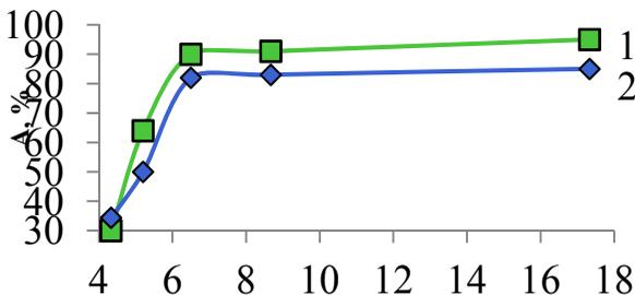
Figure 2 - Dependence of the softening efficiency of the model solution on the consumption of 5/6 aluminum hydroxychloride (lime dose mg-equivalents/dm<sup>3</sup>: 82.2 (1), 123.8 (2))
