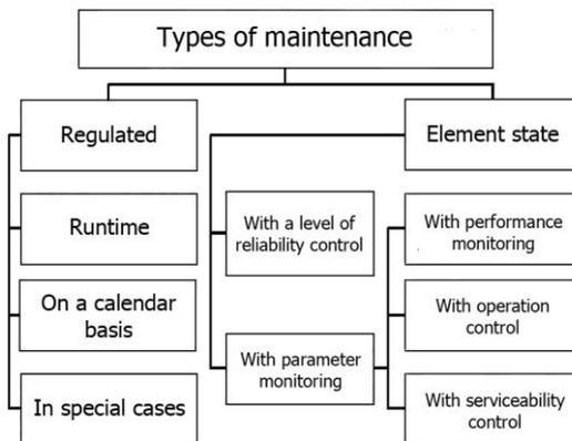
Fig. 1. Classification of maintenance types
