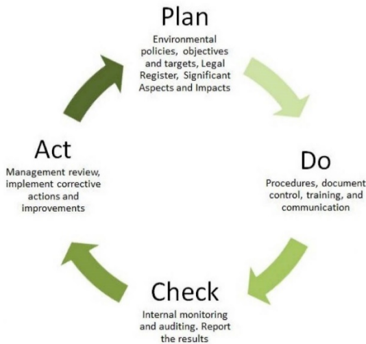
Fig.1. Schuhart-Deming cycle of SEM
