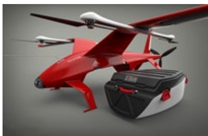
Fig. 2. Model of the designed hybrid UAV Airbus «Zelator-28» [2]
