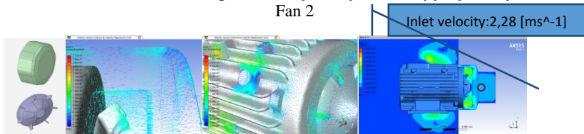
Fig. 8 Result of CFD for Velocity for fan 2 / fan cover 1
