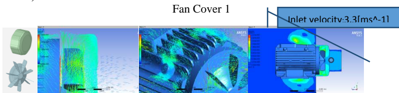
Fig. 10 Result of CFD for Velocity for fan 1 / fan cover 1
