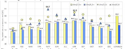
Figure 3. Equivalent sound level from the period of one day, one month and year for day and night measured at one measurement point
