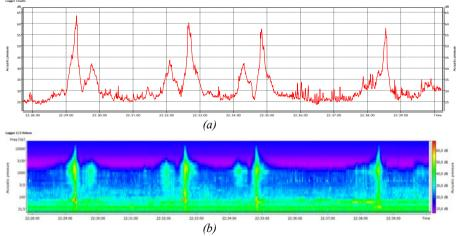
Figure 2. Time history of the registered noise level of aviation noise (a) along with the identification of acoustic events (b) This collection of information:
