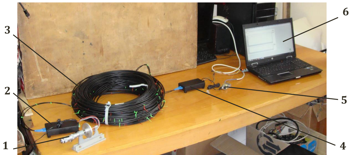
Figure 3. Experimental research of the HFOS with measuring and data analysis system: 1 – sensor with measuring transducer; 2,4 – transducer electrical digital code to optical digital code and optical digital code to electrical digital code with digital controller; 3 – optical fiber; 5 – operation control systems of control mechanical parameters of the aircraft unit.
