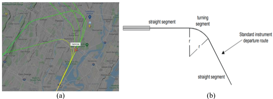
Figure 3. Approaches to track description: (a) example of point-to-point track (by flightradar24.com); (b) required navigation performance by ICAO DOC 9911
