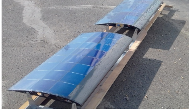
Fig. 2. An experimental fragment of a wing with applied photocells
