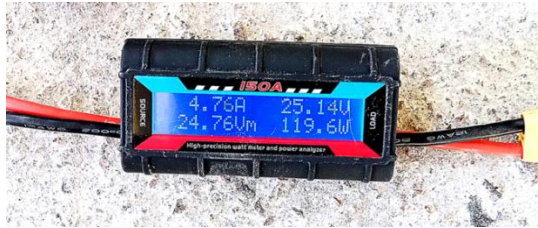
Fig. 5. Wattmeter with maximum power mode parameters
