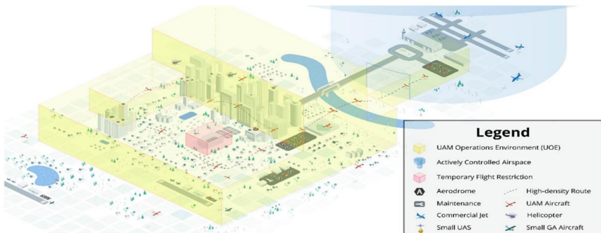
Fig. 2. The air traffic integration between usual air traffic system (airports and airlines) and the Urban Air Mobility
